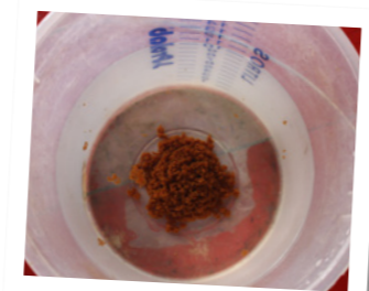
After a while, all the impurities settle to the bottom of the bucket. Potable water can now be scooped out.
