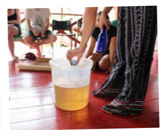
Four grams of powder are enough to purify 10 litres of water. The whole thing is stirred for a few minutes.
